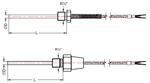
**VR07** Type resistance thermometer has a simple flat type structure with fixed cable. Cable length must be specified in the order. There is a pipe at the end of the cable. This pipe can be given in "L" length in different diameters. In standard production, VR07 cable outlet is springy.
