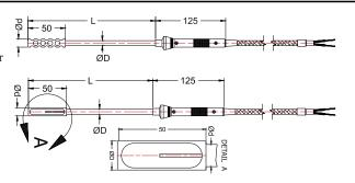
**VR12** Type resistance thermometer 43650 is electrical or M12 socket. Standard raccord size is 1/2". For detailed and different types of choices, please check our VR12 type resistance thermometer catalog in Resistance thermometers section.
